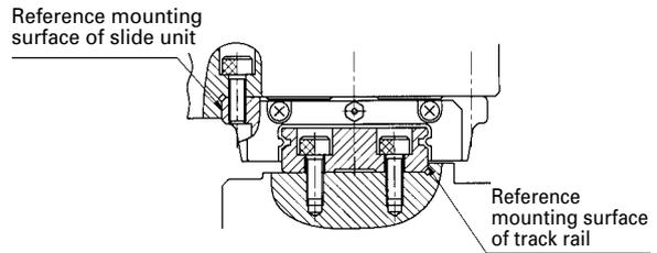
The reference mounting surface of track rail is made opposite to the standard side. The accuracy of dimension N including parallelism in operation is the same as that of standard specification.
