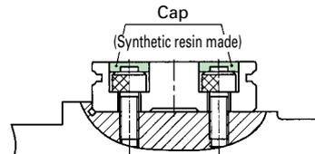
Specially prepared caps for track rail mounting holes are appended. These caps cover the track rail mounting holes to improve the sealing performance in the linear motion direction. Aluminum caps are also available. Consult for further information.
