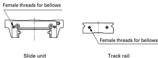
Female threads for mounting bellows are provided on the interchangeable slide unit or the interchangeable track rail. For details of related dimensions, see Table 6.
