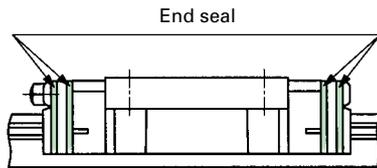
Double end seals are provided on the slide unit of assembled set of interchangeable specification or non-interchangeable specification for more effective dust protection. For the total length of the slide unit with double end seals, see Table 7.
