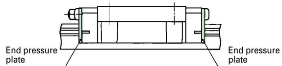
End seals at both ends of slide unit are replaced by end pressure plates (not in contact with the track rail) to reduce frictional resistance. This specification is not effective for dust protection.
