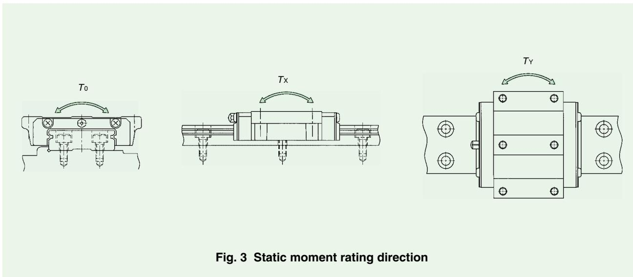
Fig. 3 Static moment rating direction
