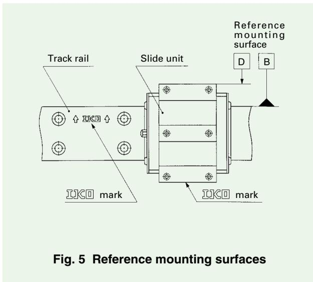
**Fig. 5 Reference mounting surfaces**
