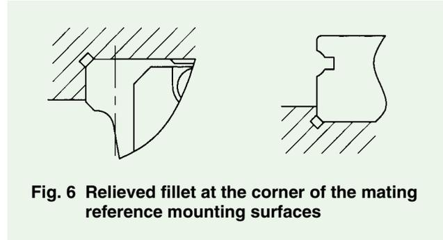
**Fig. 6 Relieved fillet at the corner of the mating reference mounting surfaces**
